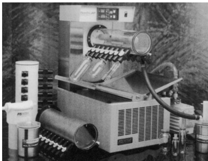
Fig. 2.8.1. Freeze-drying plant for flasks and bottles, 16 connections 1/2 in, titanium condenser for maximum 3 kg of ice in 24 h, con-
