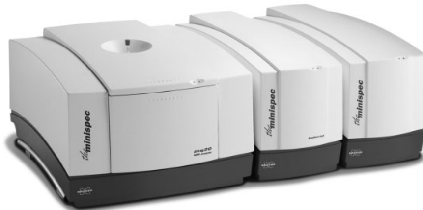
Fig. 1.49. NMR analyzer, the >Minispec< mq series, measurement range -100 to +200 °C (Bruker Optik, Rheinstetten, Germany)
