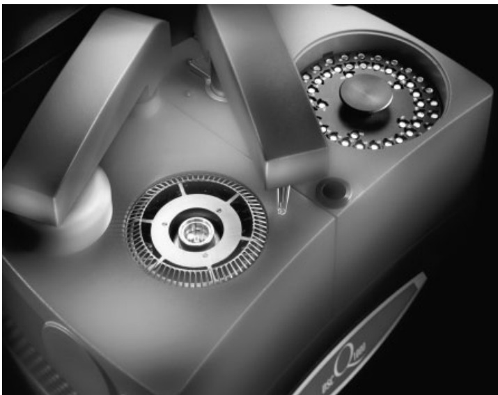
Fig. 1.45.2. Automatic sample manipulator. The left robot arm covers cell and oven during operation, the sample arm positions the probe pan. (TA Instruments, Inc., New Castle, DE, USA)
