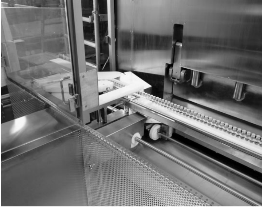
Fig. 2.72. Automatic loading system in front of a freeze-drying plant with loading door (slot door). (Steris GmbH, D-50354 Hürth, Germany).
