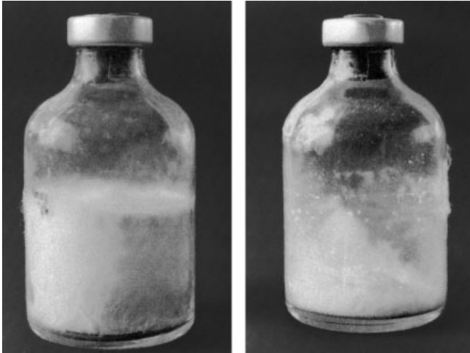
Fig. 3.9. Photographs of two vials with freeze-dried factor VIII. Left, frozen in \text{LN}_2 ; right, frozen on the shelves of the freeze-drying plant (Figure 8 from [3.23])
