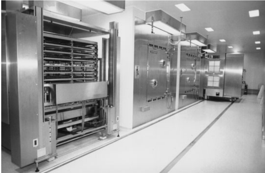
Fig. 2.73.2. Sterile wall with two freeze-drying plants (10 m 2 shelf area each), one loading storage (front) with 10 divided shelves and one unloading storage (behind transfer cart).
