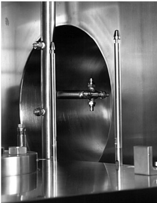
Fig. 2.64.1 (a and b). CIP spray rod in the drying chamber. Spray rods are installed at the four corners of the drying chamber. The 90° flat spray jets are placed at different positions and heights on these rods. Part (a) also shows spray jets over which the connecting pipe between the chamber and the condenser as well as the valve are cleaned. The positioning of the jets is determined over computer animation to achieve the highest possible degree of cleaning: >99%. (Photograph Steris GmbH, D-50354 Hürth, Germany).
