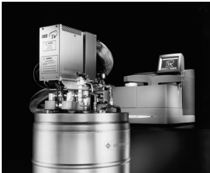
Fig. 1.46. Modulated DSC® apparatus, Model Q 1000, using the details of Figs.1.45.1 and 1.45.2 (TA Instruments, New Castle, DE, USA)
