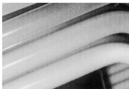
Fig. 2.18. Coils in a condenser covered by ice, observed through a window during two freeze-drying processes. Left: smooth, solid surface. Right: porous, snow-like surface, which occurs
