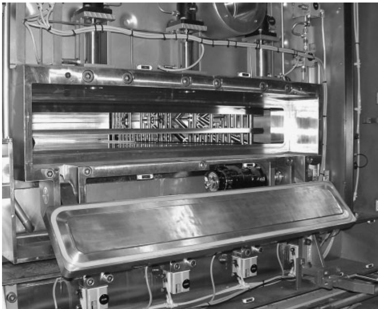
Fig. 2.12. Rectangular chamber, steam-sterilized, with a small loading door in the main door, which can be designed to open either
