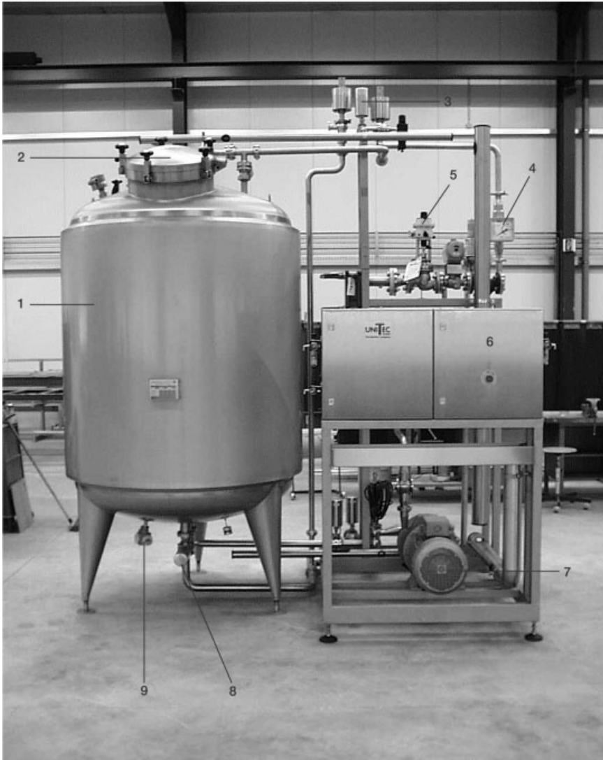
Fig. 2.65. CIP skid. 1, Tank; 2, manhole; 3, venting filter; 4, flowmeter; 5, safety valve; 6, control cabinet; 7, circulation pump;
