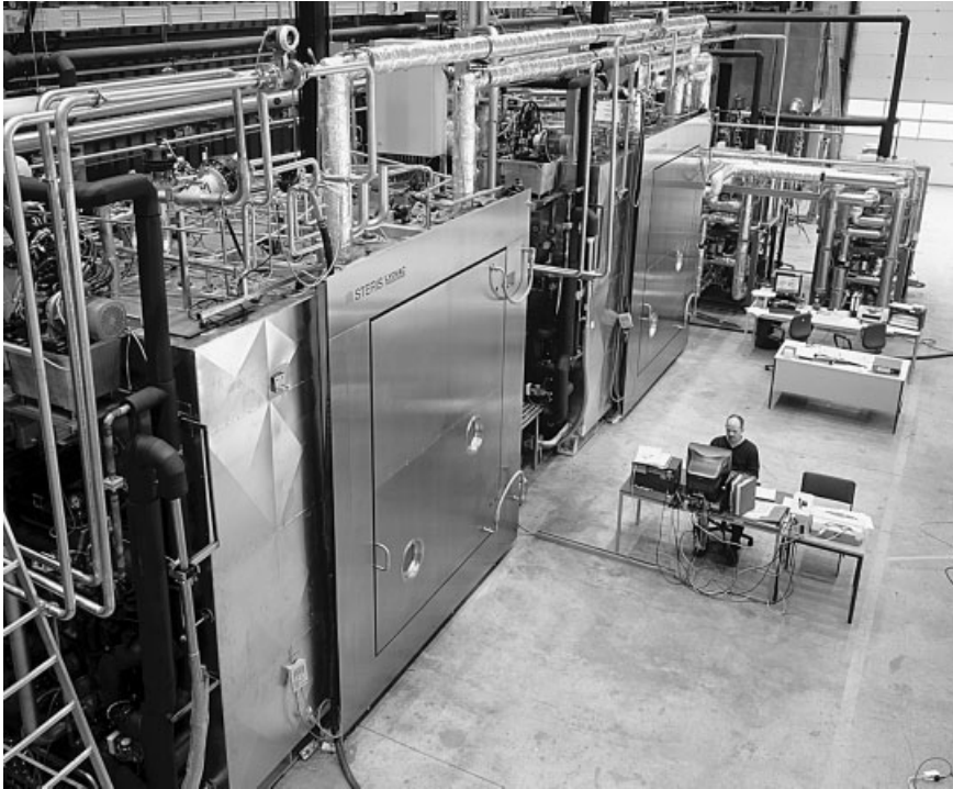
Fig. 2.71.1. Steam sterilizable-production plant with two LYOVAC® GT 500-D. The condensers are directly flanged to the chambers
