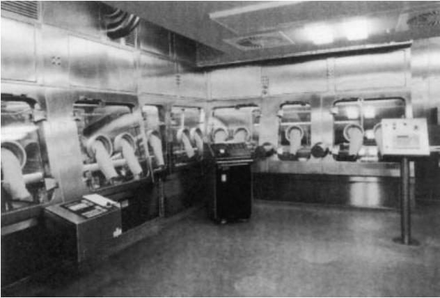
Fig. 2.74.1. Automatic loading and unloading system (ALUS), completely enclosed in isolators, for vial transportation. (Steris GmbH, D-50354 Hürth, Germany).
