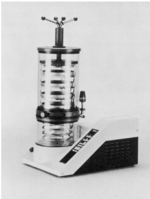
Fig. 2.10. Freeze-drying plant of the type in Figure 2.9(a). 1600 cm 2 temperature-controlled shelf area stoppering device for vials on four shelves, valve between chamber and condenser, for BTM and DR measurements, freezing is possible between the condenser coils or in the shelves if they are cooled and heated by brine from a thermostat, T_{co} down to -55\text{ }^{\circ}\text{C} (LYOVAC® GT 2, Steris GmbH, D-50354 Hürth, Germany).
