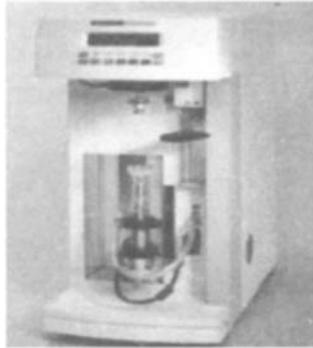
Fig.2.21 A thermogravimeter (Pyris 1, Perkin Elmer Comp.)
