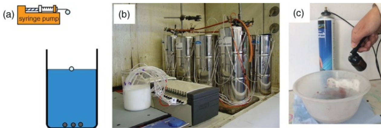
Figure 1.7 (a) The diagram shows a solution/emulsion/suspension injected into liquid nitrogen. (b) The photograph shows parallel injection into liquid nitrogen using a peristaltic pump. In this case, a milky oilinwater emulsion is injected into liquid nitrogen contained in a few dewars. (c) Illustration of a solution/suspension/emulsion being sprayed into liquid nitrogen using a simple aerosol sprayer. (Note: This photograph is for illustration only with the plastic bowl. For the experiments, an openmouthed dewar is always used.)
