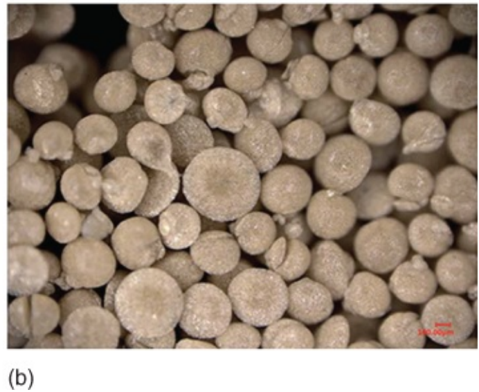
Figure 7.16 Porous graphene spheres by electrospaying into a cryogenic liquid. (a) The schematic preparation process. (b) The optical microscopic image of graphene spheres.
