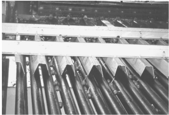
Figure 20.2. Cherries travel down the sizer of diverging rollers lubricated with cold water.
