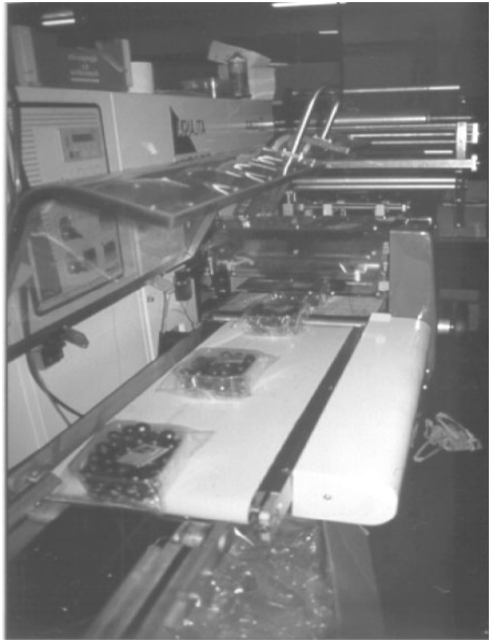
Figure 20.3. Horizontal flow-pack wrapping of sweet cherry punnets.
