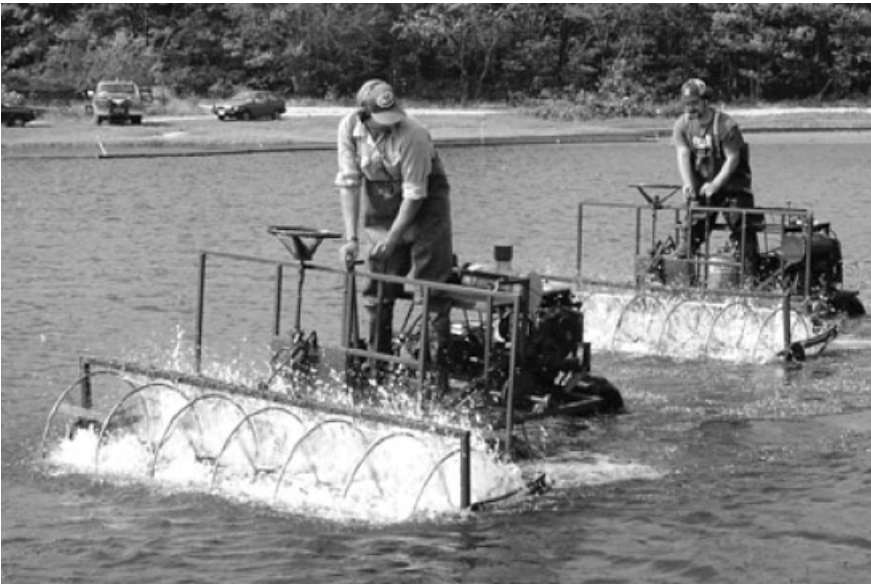
Figure 21.1. Water reels dislodging fruit from vines.
