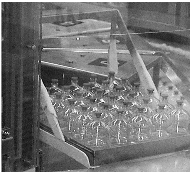
Figure 2.3 The vials filled with product are placed in baskets and taken to the infeed station of the freezing system. The basket is lowered automatically into the \text{LN}_2 bath and is transported step by step through the system. At the exit station, the basket is lifted automatically out of the \text{LN}_2 bath and manually loaded on to the shelves of the freeze-dryer that have been precooled to <-60^\circ\text{C} . The product temperature when taken out of the freezing bath is approximately -80^\circ\text{C} . (Baxter SA, B-7860 Lessines, Belgium.)
