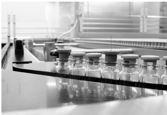
Figure 2.101 Vial with installed antenna is placed on the ALUS conveyor belt. (Tempris Sensor Technology, IQ Mobil Solutions GmbH, D-83607 Holzkirchen, Germany.)
